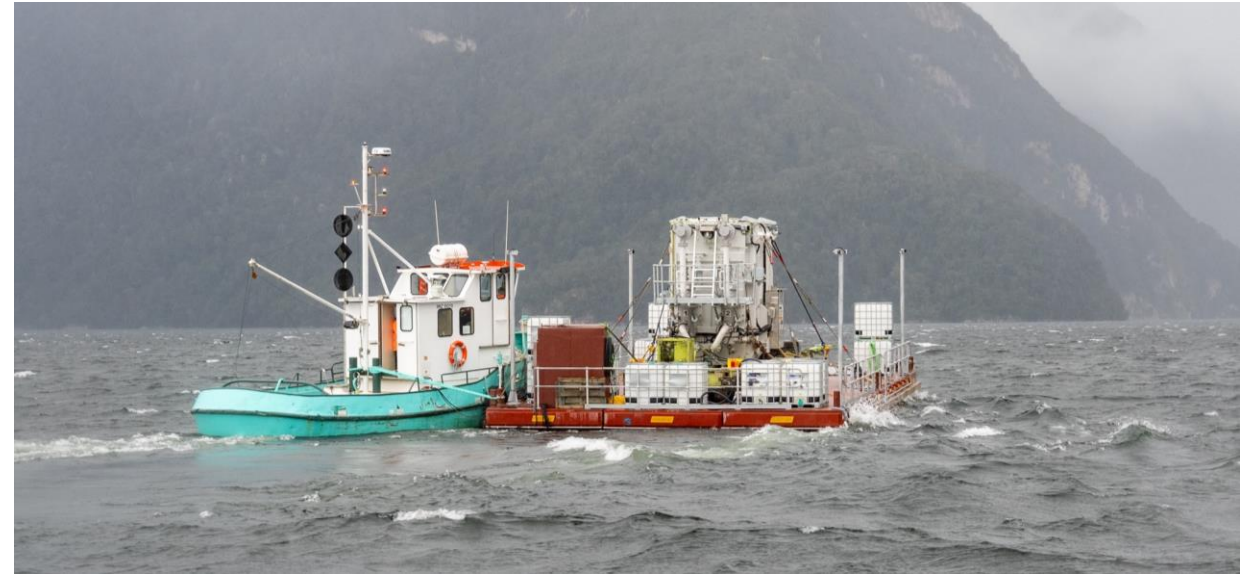
Transportation of a transformer across Lake Manapōuri
